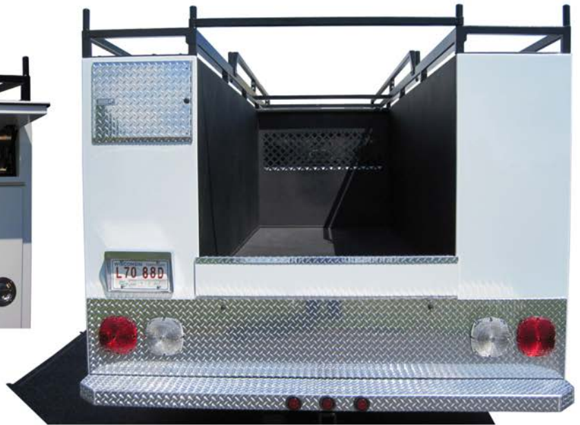
Rear Cargo Compartment 48.00" W x 120.00" D Flip-Down Rear Tail Gate
