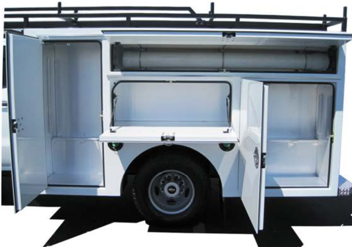
Driver's Side Body Compartments Front Side: 29.00" W x 56.00" H Over Wheel: 46.00" W x 33.00" H Over Wheel Long: 82.00" W x 11.00" H Rear Side: 33.00" W x 41.00" H
