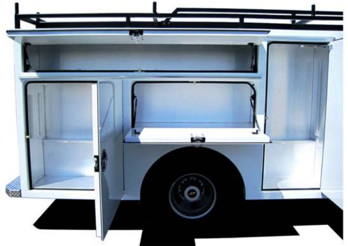
Rear Cargo Compartment 48.00" W x 120.00" D Flip-Down Rear Tail Gate
