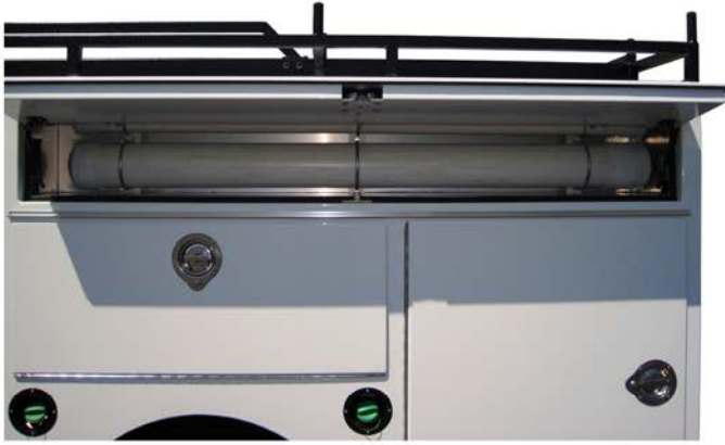
Schedule 40 PVC Storage Tubes Access tubes through rear upper diamond plate door opening
