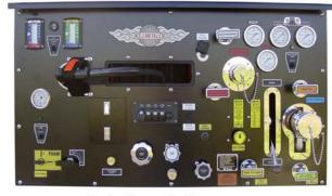
Twin Pump Performance: 8 GPM @ 2800 PSI - (tested) Darley 1-1/2 AGH - 126 GPM @ 129 PSI - (tested)
