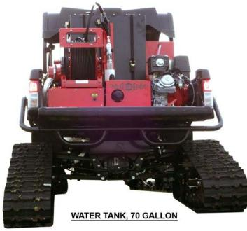
The water tank shall be constructed from aluminum, welded and power coated inside and out.
