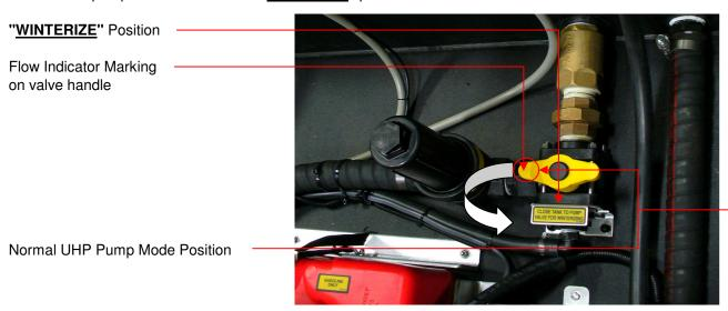
2 Attatch provided hose section to "WINTERIZE" port fitting on pump control panel .
