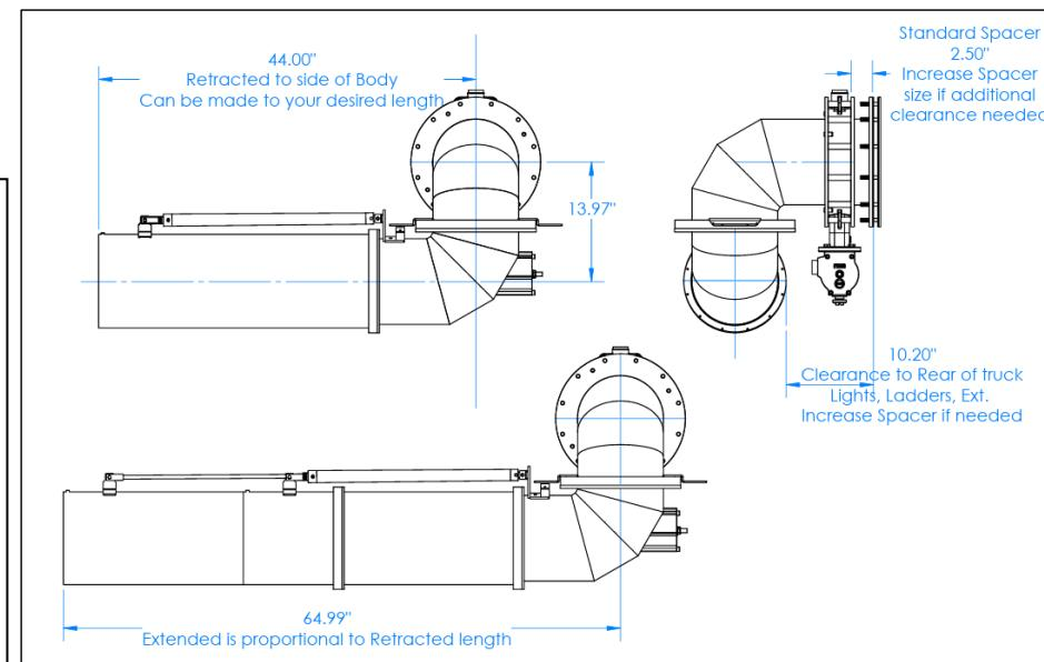
**Highlights:** Lightweight, durable aluminum body, adjustable speeds for chute actuation, powder coated options, air or manual extension, 180-degree swivel capabilities, chute tubes sealed on both ends to prevent leaks and to prevent contamination to sliding mechanism.
